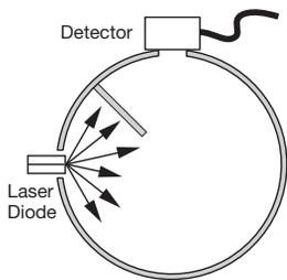
Collimated Laser Beam Power Measurement
