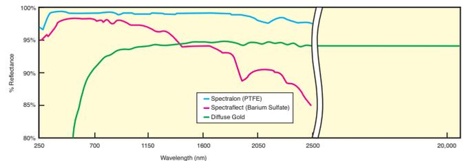
Our integrating spheres are available with PTFE (spectralon), barium sulfate (spectralect), and diffused gold sphere materials.
